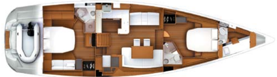
3 cabin version : owner's aft cabin and 2 transformable cabins forward. Optional forward cabin.
